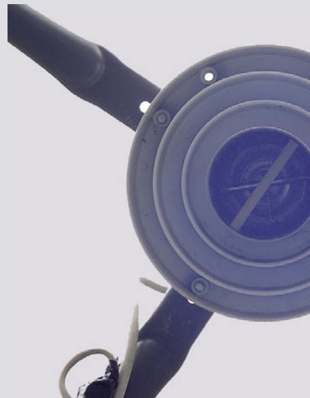
▲ A look inside the feed opening: clearly recognizable is the dielectric that is necessary for reception of circularly polarized signals. Remove it and you have linear reception.
